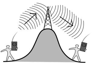
downlink is at a higher or lower frequency from the uplink respectively.
